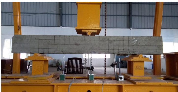
CIVIL-22: 1.5 METERS SPAN REINFORCED CONCRETE BEAM TESTING ON 100 TON LOADING FRAME IN STRUCTURAL ENGINEERING RESEARCH LABORATORY
